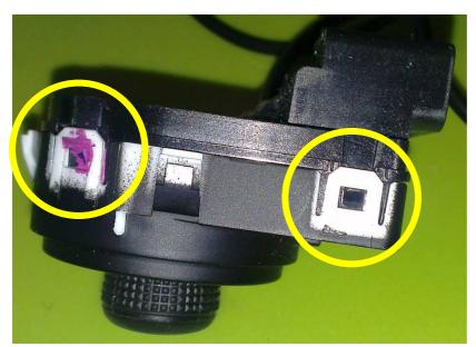
To open the mirror switch you must release the small plastic pins with a normal small screwdriver. Two on both sides.
