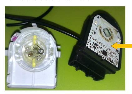
Now you have to take out the pcb (orange arrow). Just plug it carefully upwards out of the mirror switch (the black wire in the back of the picture won't be there on your mirror switch). It should look like this:
