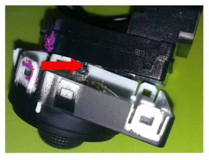
After that just pull apard both sides. Inside you will find a small spring and a metal shell, which is pulled over the spring (red arrow).
