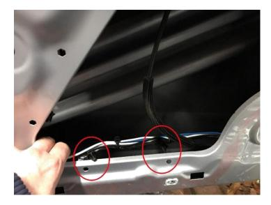
Unclip the cable harness (red circles) and attach the new cable to the old cable harness.
