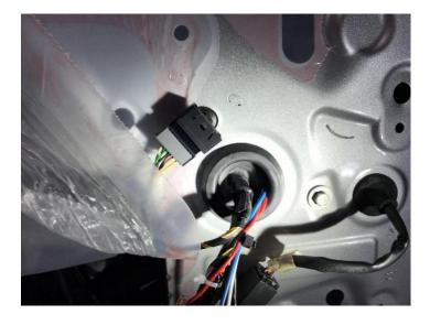
Remove the protective film at the bottom and fold it up, route the cable through the rubber seal into the interior of the door.
