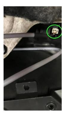
Connect the plug to the mirror switch and test the function. If everything works, the door trim can be reinstalled.
