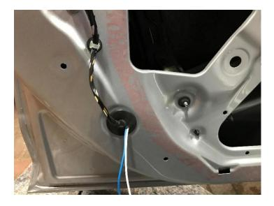
Route the cable through the rubber seal.
