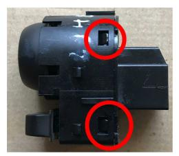
To open the switch, the small noses must be clipped out (red circle), on each side there are two of them. After unclipping the two parts pull apart.
