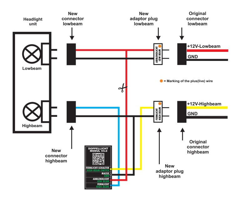
The wire colours are only for a better view on the schematic and are different to the location you want to install it.
