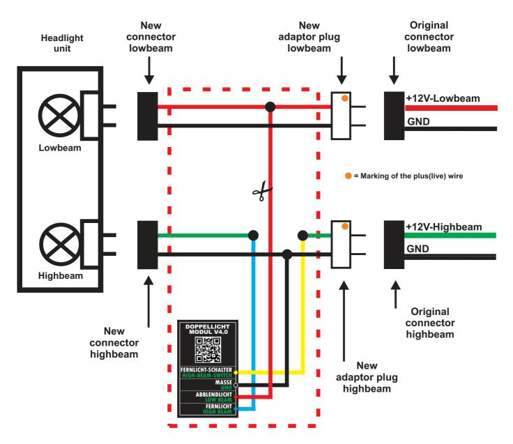
The dashed area (red) shows the connections already done by me. It should only show how the wiring was done. The wire colours are only for a better view on the schematic and maybe different to the location you want to install it.
